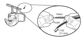
2.5B Insert the wires connected to the white safety sensor wires to the white terminal on the garage door opener. Insert the wires that are connected to the white/black safety sensor wires to the grey terminal on the garage door opener.
